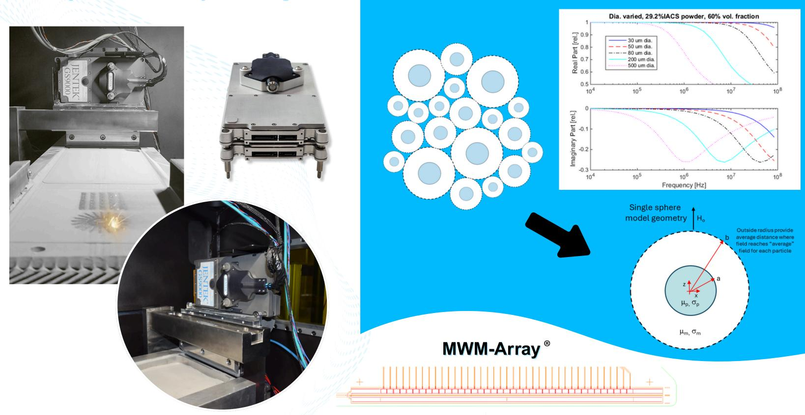
In-situ eddy current sensing that keeps up with process speed JENTEK GS9000<sup>®</sup> instrument installed on LPBF recoater
